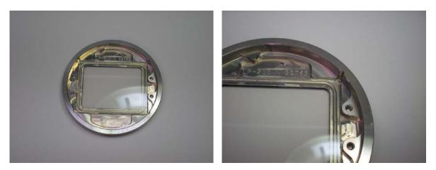
Window Glass – Sealing the viewing window glass presents a bit of a challenge, as two materials with different temperature coefficients of expansion must be joined together. A silicone adhesive with a moderate Shore A hardness of 30 and a -60C
