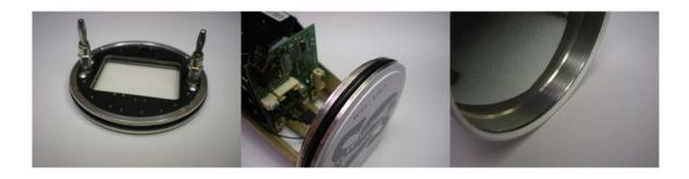
Front and Back Plate to Camera Tube Seal – Sealing the window face plate and the rear plate to the camera housing tube is accomplished using -45C to +120C temperature rated, Shore 65 hardness o-ring seals. The o-rings are greased with a -40C to +95C temperature rated silicone lubricant to provide an air tight and water tight seal. The o-ring seals mate with the precision machined surfaces on the inside front and inside rear of the camera housing tube.
