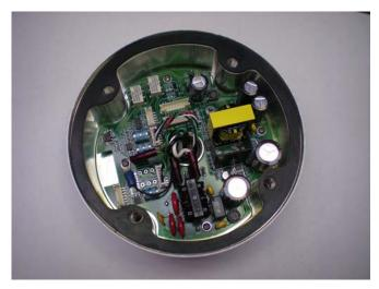
Power Supply Base Seal – The power supply base seal was actually pretty straight forward to implement. Since the main camera base structure is very heavy duty, large bolts could be used to apply the force necessary to get a highly reliable seal. A special laser cut gasket is used to seal both the mounting rim and the mounting bolts.
