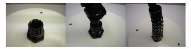
Bottom Egress Cable Seal – A water tight integrated cable seal and strain relief was used to seal the cable exit point on the bottom of the camera. A silicone sealant is used to seal the strain relief to metal housing joint. The strain relief provides a water tight seal around the cable itself.
